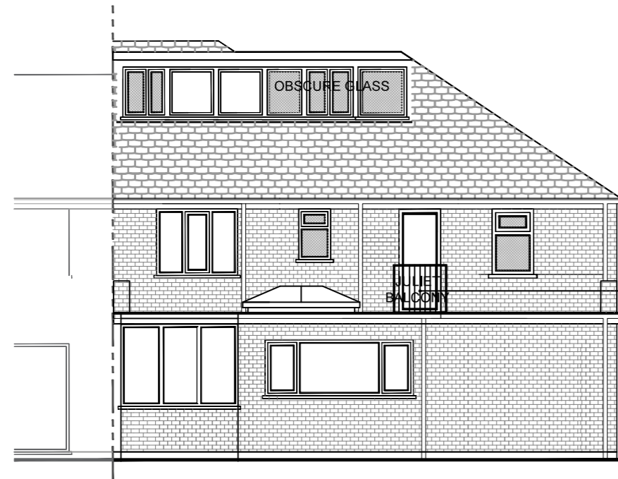
AS BUILT REAR ELEVATION
